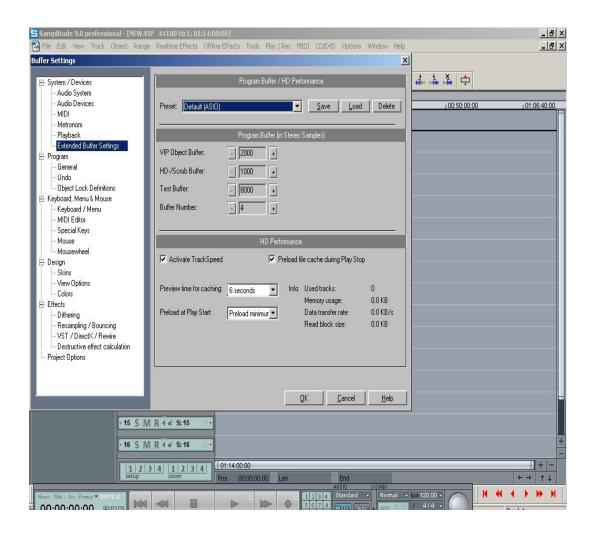
7. On the main screen, record enable a track and select the Audio drop down to map what channel from the Multimix will be sent to this track. Right click on 'In' and select the Multimix input you would like to use.
