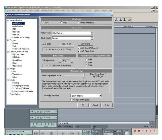
5. Then in System/Devices under Audio Devices, enable the Multimix channels. The first 4 channels are automatically activated, so the rest will also need a check mark which will allow you to record using these channels on the mixer. (see the graphic on the next page)
